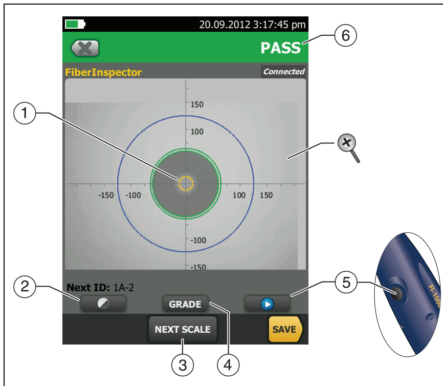
Figure 40. FiberInspector Image with Manual Grading Selected
